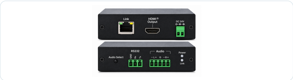
Receiver: LINK, HDMI OUT, 24 V DC, RS-232 and audio
